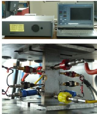
Figure 11. ACPD Detection on a double notched specimen
