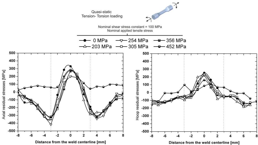
Figure 6. Welding residual stress relaxation under tension-torsion loading.
