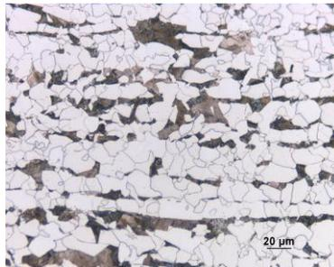
Figure 1. Microstructure in S355J2H
