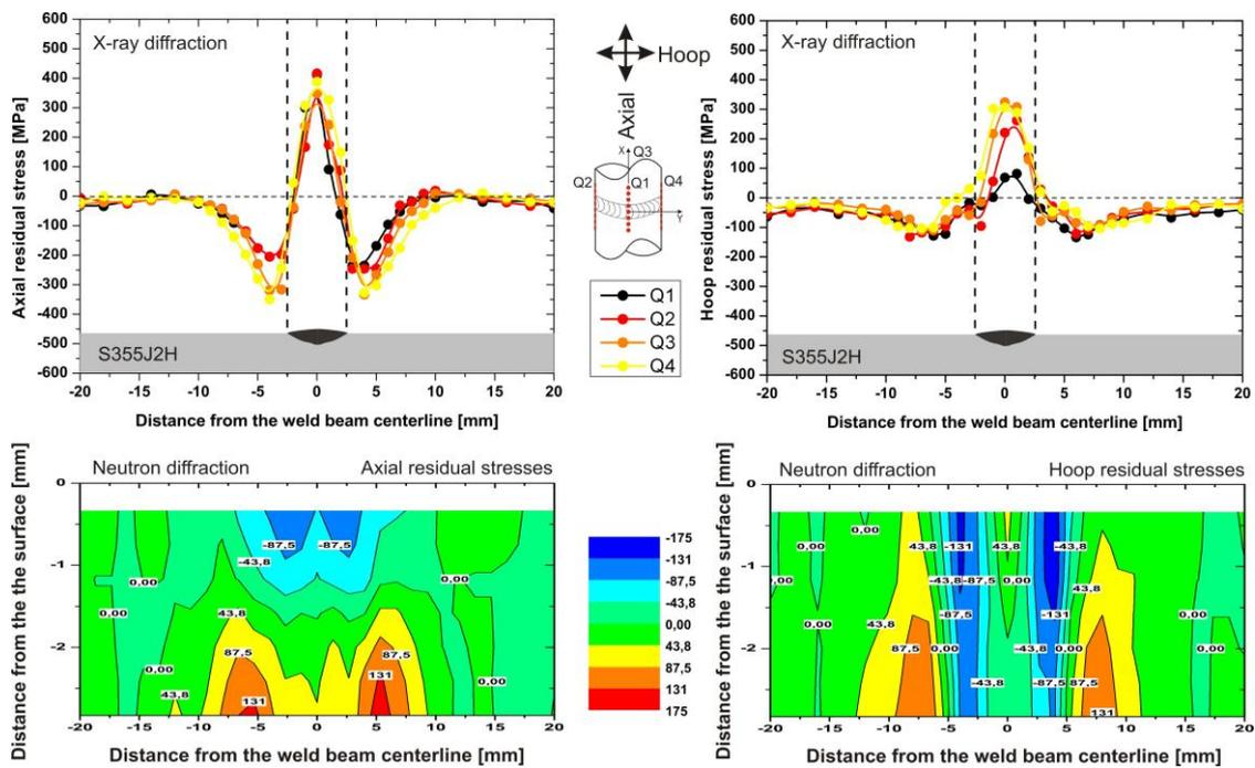
Figure 4. Residual stress field determination by means of x-ray and neutron diffraction.
