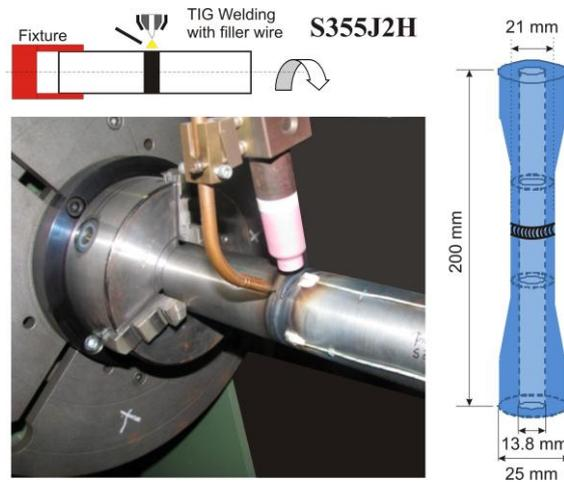
Figure 2 Representation of welding the specimen and dimension of the investigated samples in this study.
