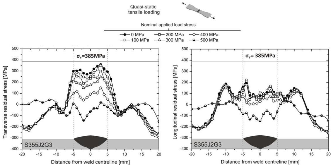
Figure 7. Welding residual stress relaxation under tension loading in flat steel specimens.
