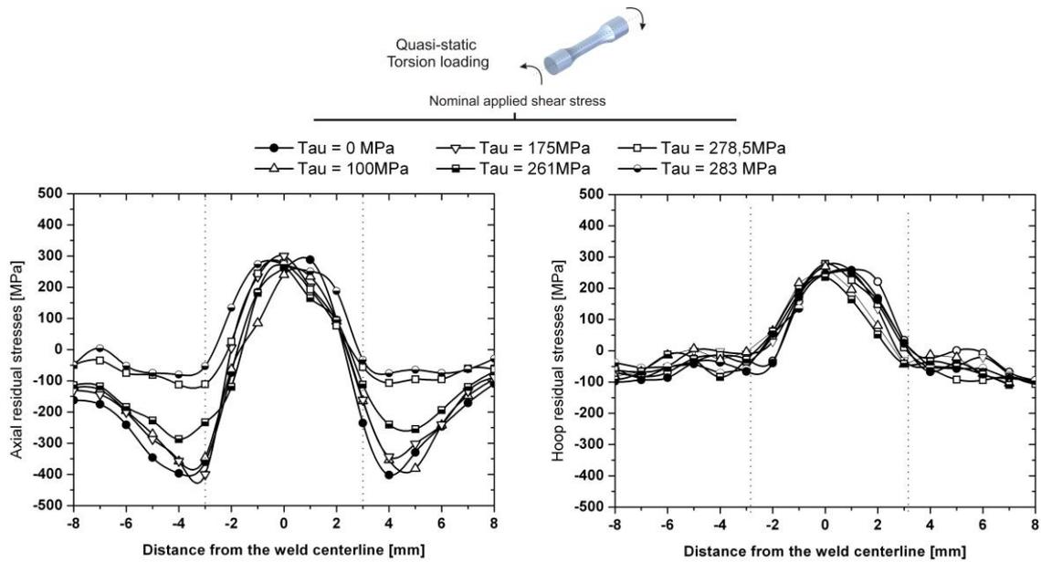
Figure 5. Welding residual stress relaxation under pure torsion.
