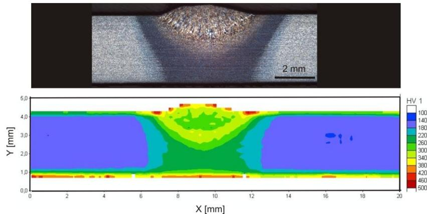
Figure 3 Cross section of the weld bead and the corresponding hardness field determined by means of UCI method.
