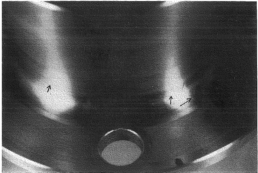
Fig 10 The tested ball-bearing ring (arrows indicate fatigue crack)
