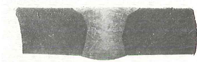
Fig 2 Typical cross-section shape of central welds in multiaxial specimens ('best' shape)
