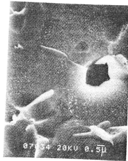
Fig. 3. Cavity inbetween ' \alpha ' and \beta grains at 750^\circ\text{C} , \dot{\epsilon} = 10^{-4} \text{ sec}^{-1} , true strain, \epsilon = 1.2 (SEM).
