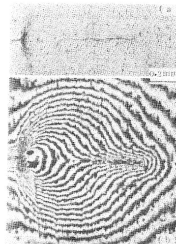
Plate 3 The crack closure behavior within plastic zone at Q_{01}=2.4 . (a) Macro-photograph and (b) Interference pattern of the plastic zone
