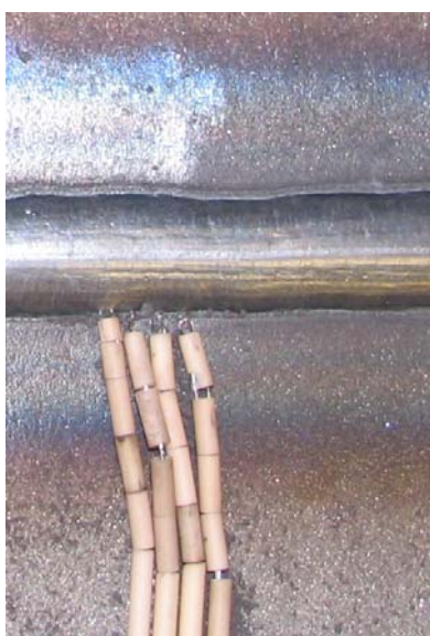
Figure 2. Positioning of the temperature sensors (left) and temperature curves for the heat treatment (right) [3]
