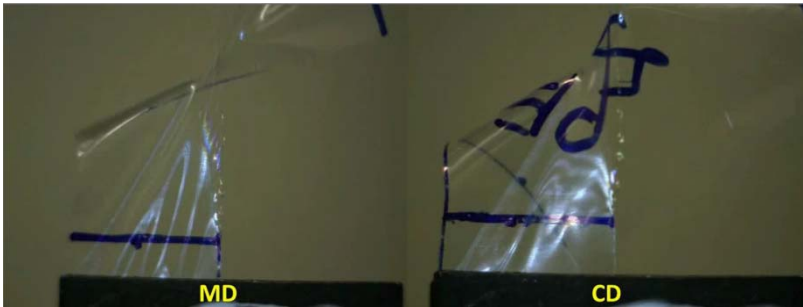
c ) final trouser tearing for MD (edge effects), extension of legs in CD
