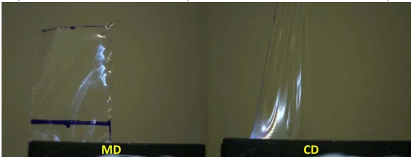
e ) finalized trouser tear test for MD, continued extension of legs in CD
