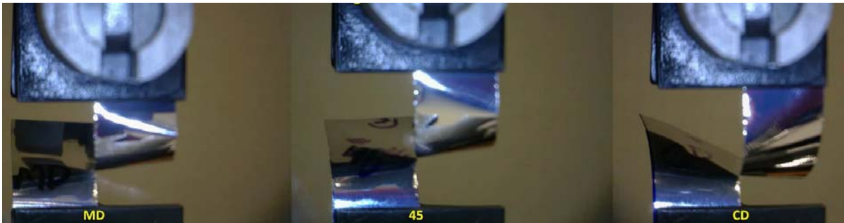
b ) continuous trouser tearing
