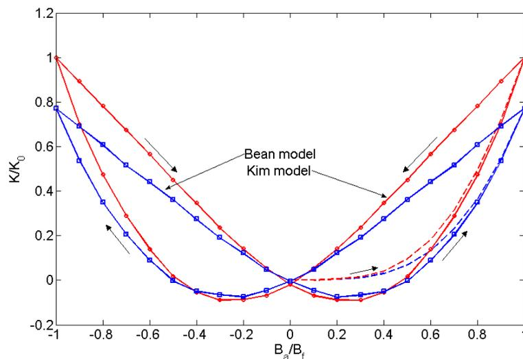
Figure 2. The development of the stress intensity factor in a full cycle applied field with maximum  $B_f$ .
