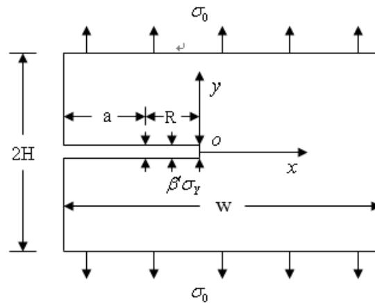
Fig. 3 Single edge crack specimen under tension
