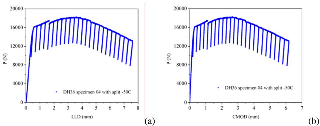
Figure 2. Experimental records of DH36 specimen 04 tested at  $-50^{\circ}\text{C}$ . a) load vs. load line displacement; b) load vs. crack mouth opening displacement.
