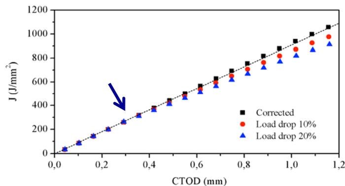
Figure 6. J-CTOD curves calculated from the records of Figure 5. The arrow indicates the position of splitting between the 5<sup>th</sup> and 6<sup>th</sup> unloading-reloading sequence.
