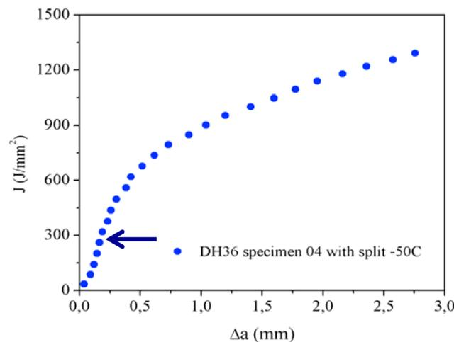
Figure 3. J-R curve of DH36 specimen 04 tested at  $-50^{\circ}\text{C}$ .
