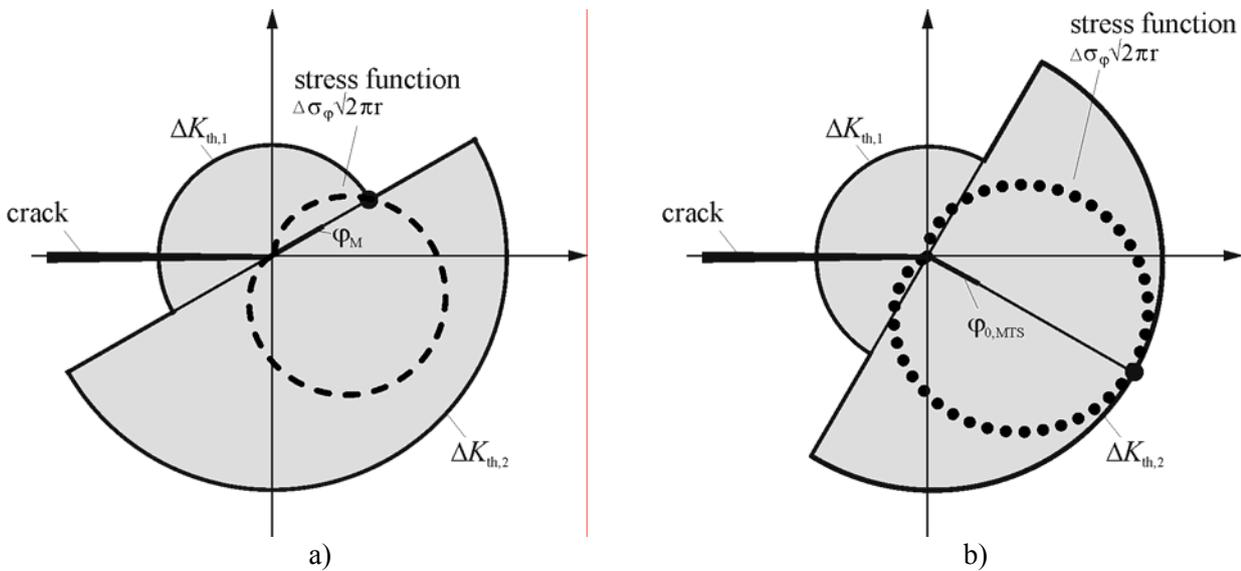
Figure 10. Occurrence and direction of fatigue crack growth for Mixed Mode loading in a fracture mechanical graded material: a) gradation angle  $\varphi_M = 30^\circ$ , b) gradation angle  $\varphi_M = 60^\circ$ .
