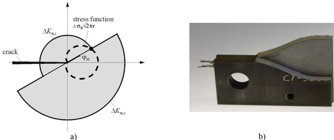
Figure 9. a) Point of contact for the determination of occurrence and direction of fatigue crack growth for a Mode I loaded crack, b) experimental confirmation of the TSSRB<sup>B</sup>-concept
