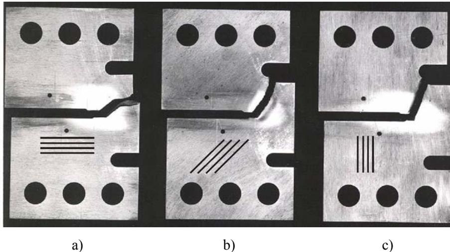
Figure 3. Aluminum alloy specimens with special rolling direction: a) in crack direction, b) diagonal, c) perpendicular to the crack direction
