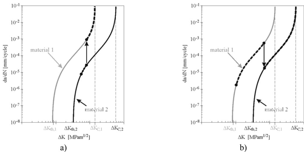
Figure 7. Schematic crack velocity curves:
