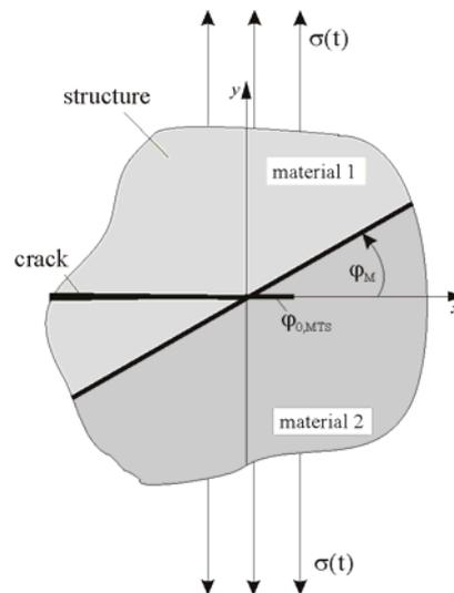
Figure 8. Fracture mechanical graded structure with gradation angle  $\varphi_M = 30^\circ$
