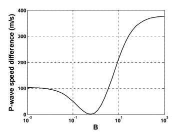
Figure 2. Dispersion magnitude (difference between high- and low-frequency velocities) as a function for parameter B. As B increases, the dispersion first decreases, reaches zero, and then increases again.
