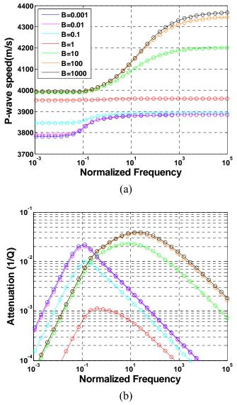
Figure 1. Frequency dependency of P-wave velocity (a) and inverse quality factor  $Q^{-1}$  (b) computed using our approximation (17) and Norris model (1) for different values of the parameter B.
