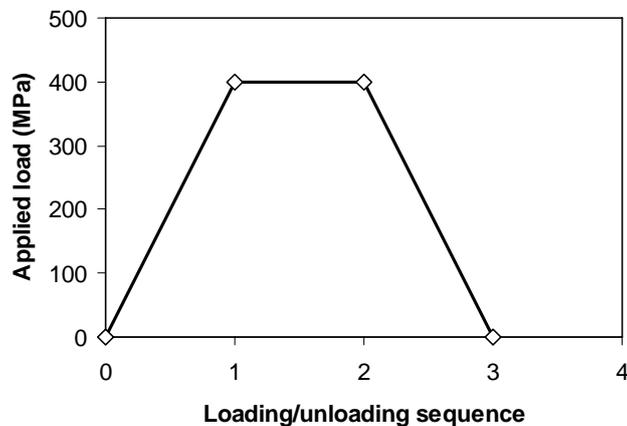
Figure 5. Loading sequence to generate residual stress
