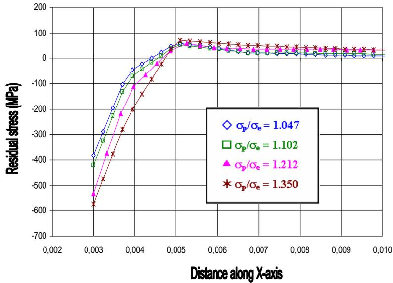
Figure 9. Residual stress along X-axis for 2024 T351 Al-alloy
