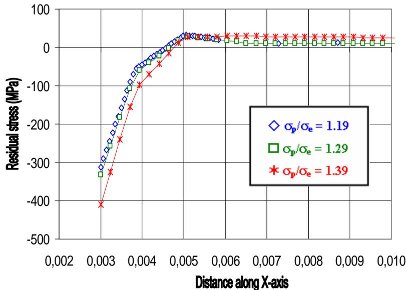
Figure 10. Residual stress along X-axis for 6061 T6 Al-alloy
