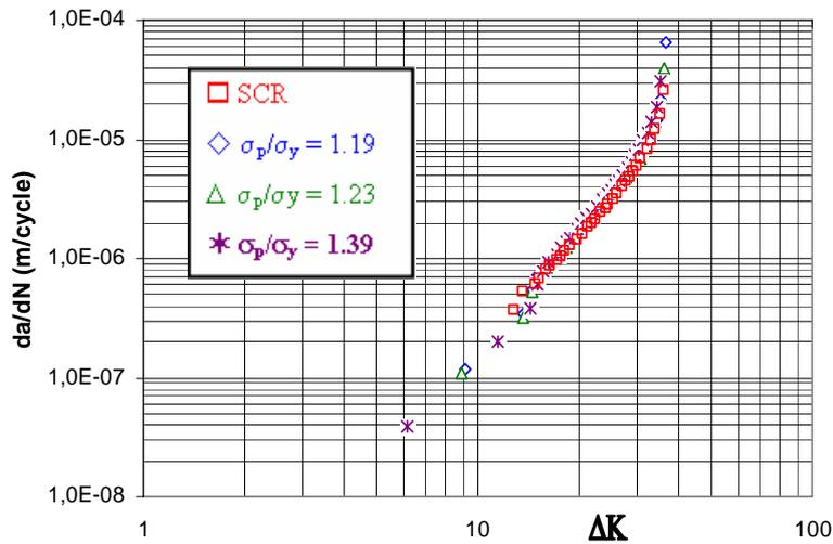
Figure 13. Preload levels effect on FCGR for 6061 T6 Al-alloy at R=0.25
