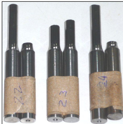
Figure 6. Photo of three non-nitrided specimens after the fatigue test.
