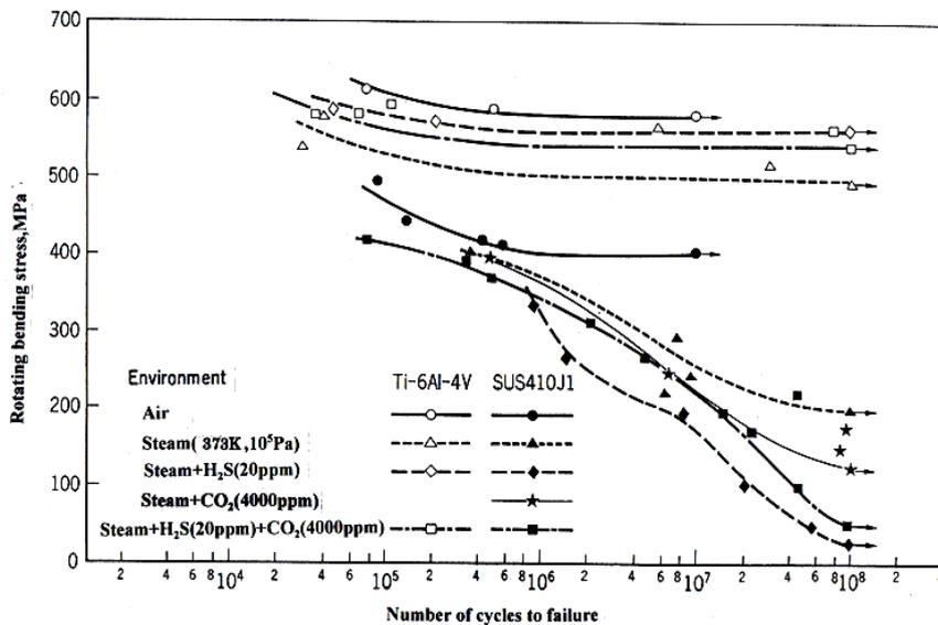
Figure1. Influence of industrial gas in steam on fatigue strength of SUS410J1 and Ti-6Al-4V[Ebara[24]].
