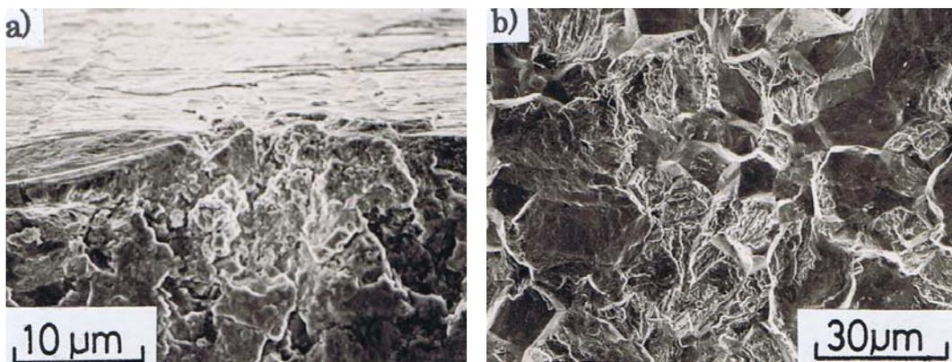
Figure 2. Corrosion fatigue fracture surface of 12 Cr stainless steel in 20ppm H<sub>2</sub>S and 4000ppm CO<sub>2</sub> in steam[Ebara[24]].
