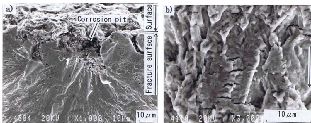
Figure 4. Corrosion fatigue fracture surface of 17-4pH T type welded joint in humid air(353K, 90% relative humidity) containing 5000ppm H<sub>2</sub>S gas [Ebara et al.[26]].
