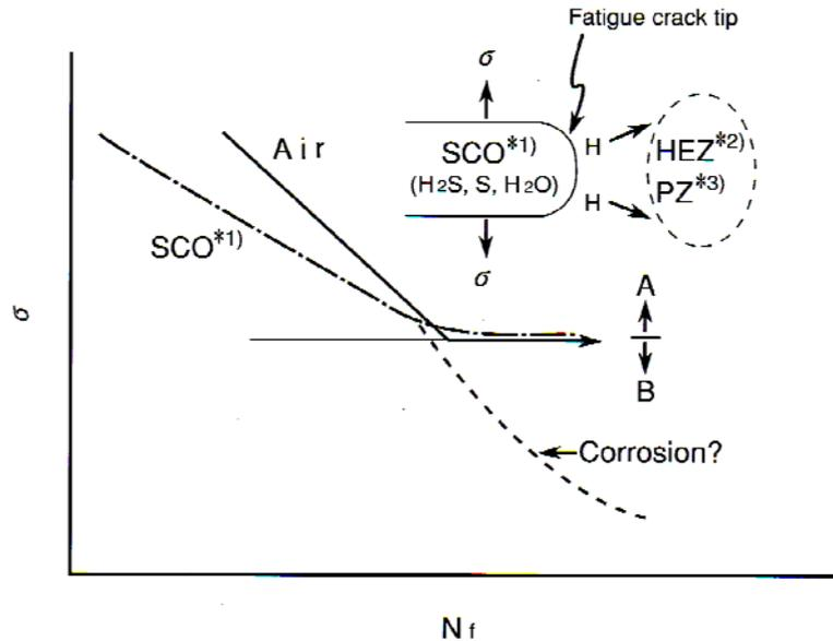
Figure 8. Schematic illustration of corrosion fatigue mechanism in sour crude oil environment[Ebara et al.[37]]. Note: <sup>\*1)</sup> SCO; Sour Crude Oil <sup>\*2)</sup> HEZ; Hydrogen Embrittlement Zone <sup>\*3)</sup> PZ; Plastic Zone
