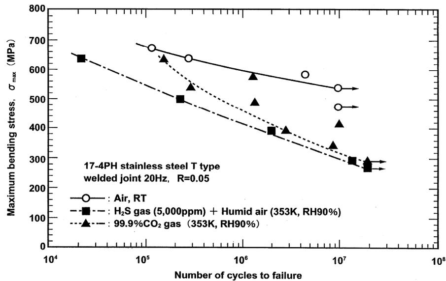
Figure 3. S-N curves of T type welded joints of 17-4pH T type welded joints in H<sub>2</sub>S and CO<sub>2</sub> gas environment [Ebara et al. [26]].
