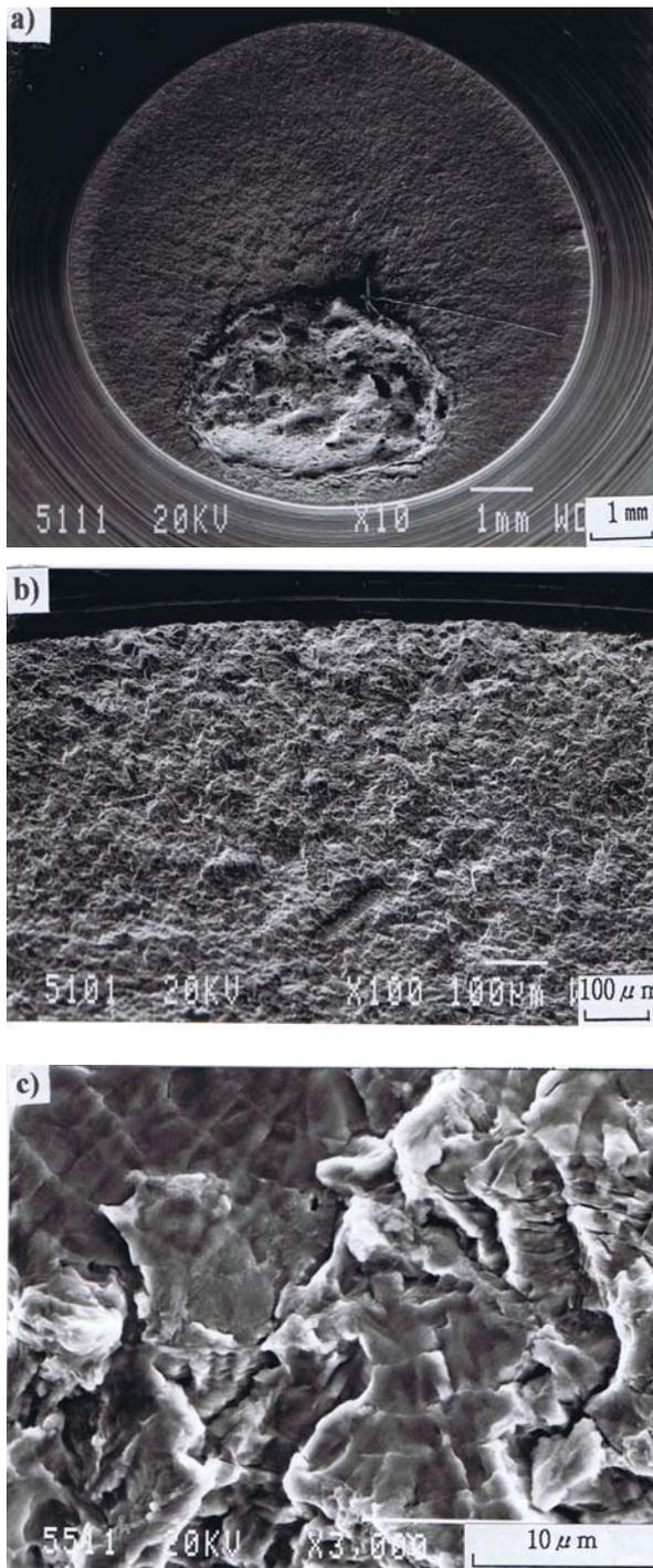
Figure 6. Corrosion fatigue fracture surface of HT50(TMCP) steel in sour crude oil ( $H_2S$ 400ppm) [Ebara et al. [37]]. round notched bar specimen 294,2MPa,  $2 \times 10^4$  cycles
