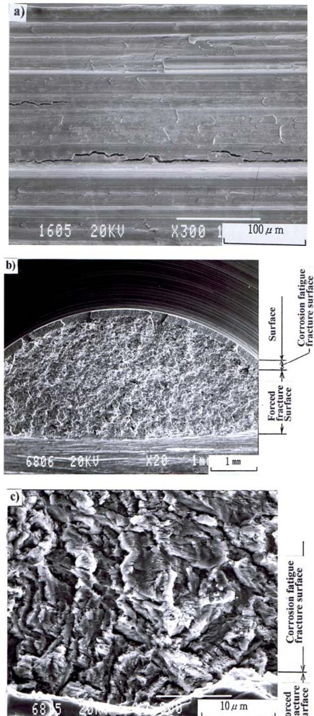
Figure 7. Surface crack and fracture surface of HT50(TMCP) steel in sour crude oil ( $H_2S$ 400ppm) [Ebara et al. [37]]. round notched bar specimen 196.1MPa, unfailed after  $1.66 \times 10^6$  cycles
