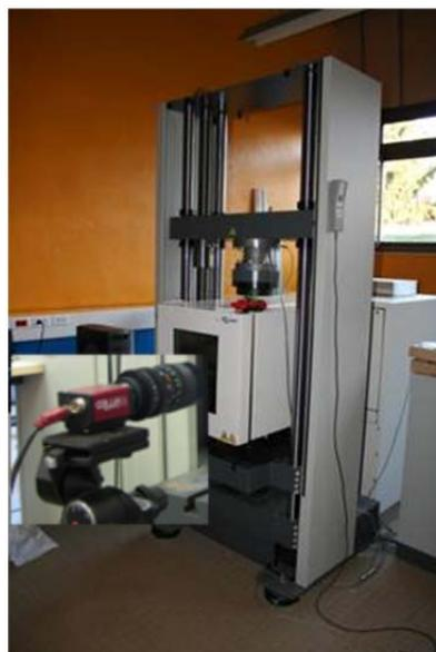
Figure 2. Zwick electromechanic machine and CCD camera
