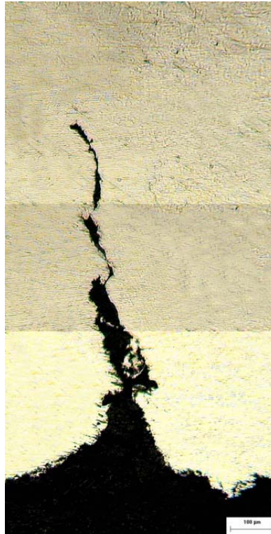
Figure 5. Photographs of; (a) Stage I crack emanating from a corrosion pit and blunt crack growth associated with inclusions for the sample in NNpH environment under Condition
