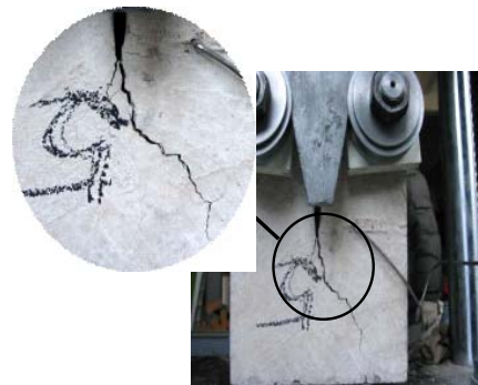
Fig.6. P vs CMOD curves of specimens with temperatures Fig. 7. Testing phenomenon of post-fire specimens
