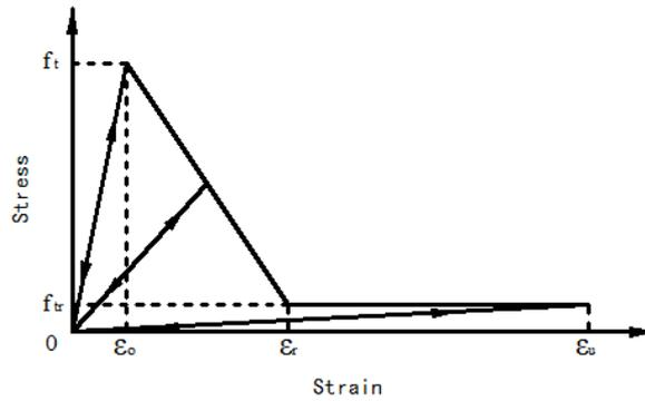
Figure 4. Bilinear damage model
