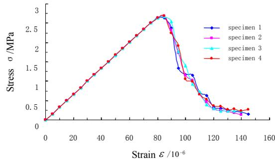
Figure 6. Stress-strain curve of RAC with 100mm×100mm×100mm
