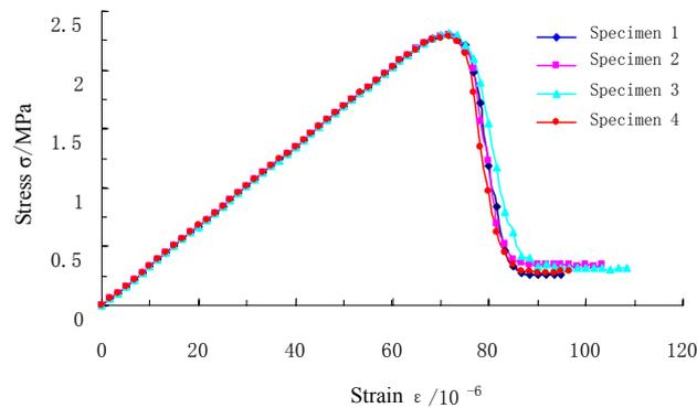
Figure 10. Stress-strain curve of RAC with  $300\text{mm} \times 300\text{mm} \times 300\text{mm}$
