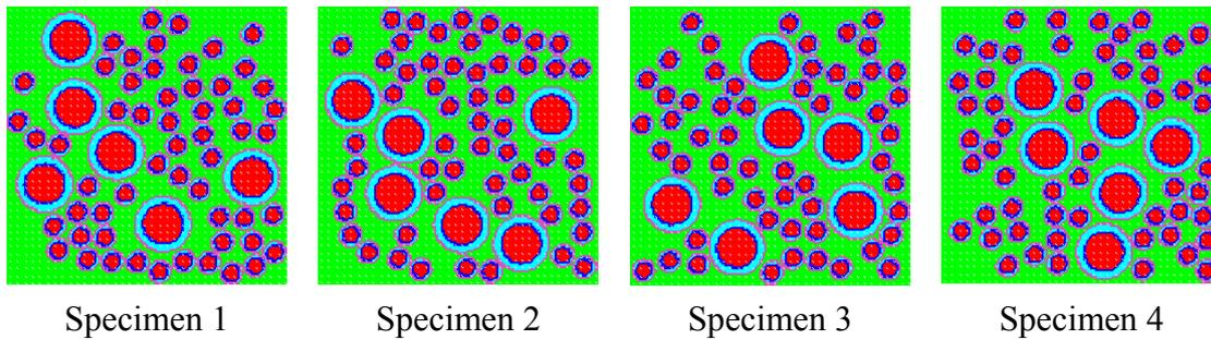
Figure 7. Random aggregate model with 150mm×150mm×150mm
