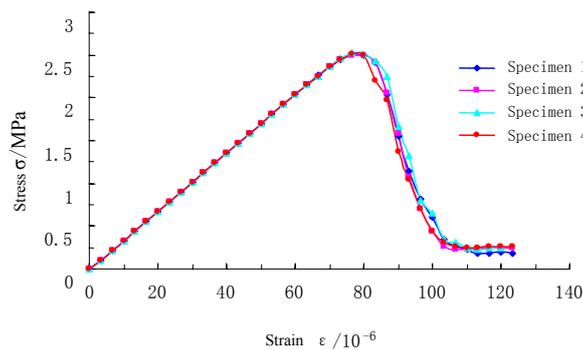
Figure 8. Stress-strain curve of RAC with 150mm×150mm×150mm
