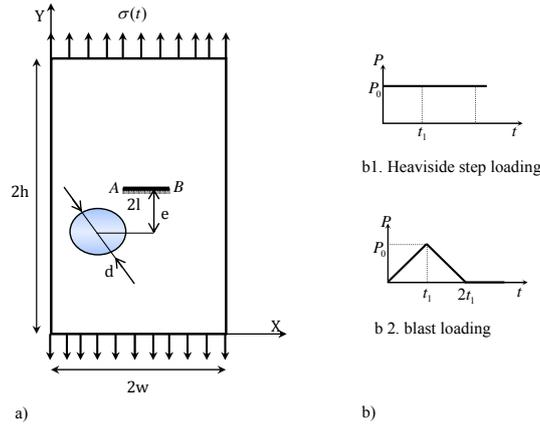
Fig.3 The validation problem: a) Cracked plate with inclusion, b) Different types of loadings.
