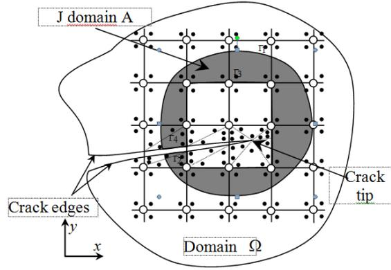
Fig. 2 Computing method of DSIF: interaction integral technique.
