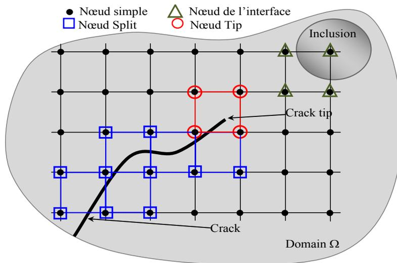
Fig. 1 Types of XFEM enrichments of the meshed domain.
