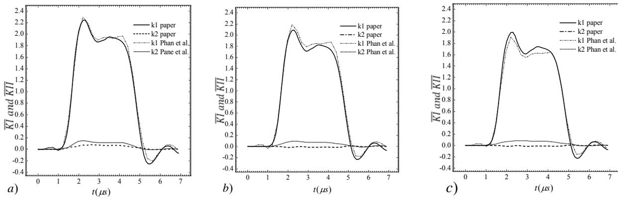
Fig.4 The plate under Heaviside step loading with different positions of the inclusion; (a)  $e = 3d/4$  (b)  $e = d/2$ , (c)  $e = d/4$ .
