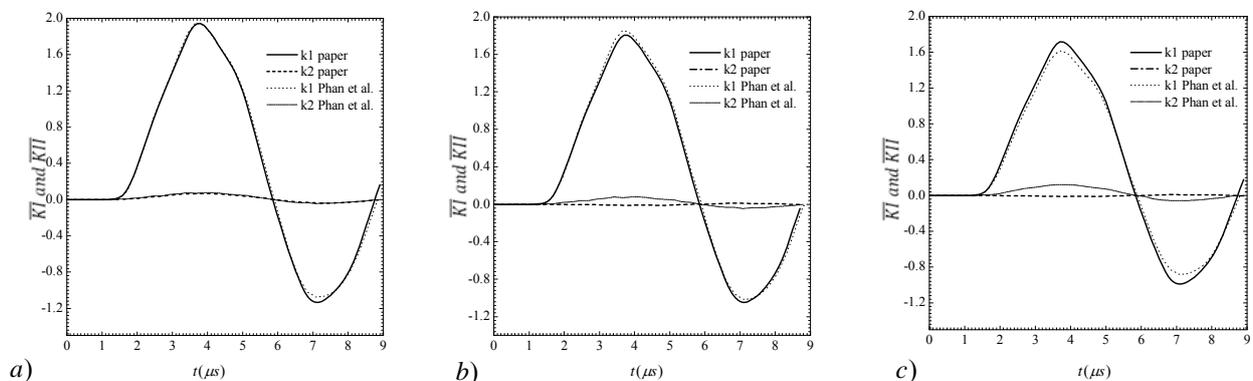
Fig.5 The plate under triangular blast loading with different positions of the inclusion; (a)  $e = 3d/4$  (b)  $e = d/2$ , (c)  $e = d/4$ .
