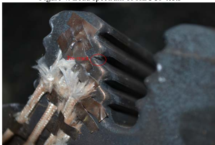
Figure 5. Pre-crack at the second tooth of the turbine disc
