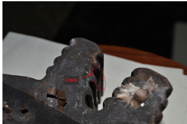
Figure 6. Macro morphology of the turbine component
