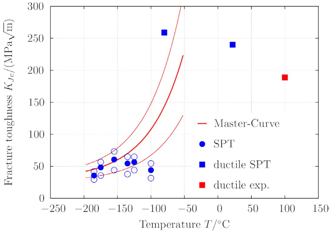
Figure 3: Fracture toughness values for the non-irradiated material JFL
