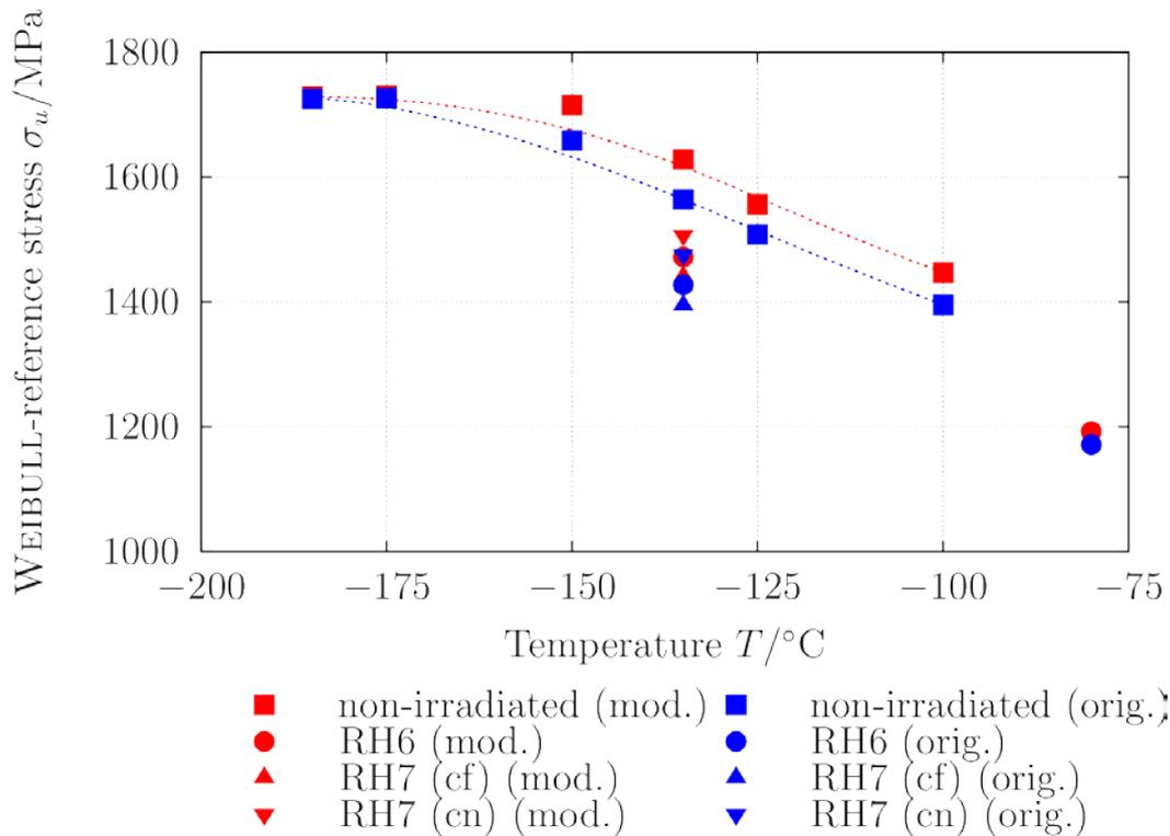
Figure 2: Weibull reference stresses identified from the SPT (material JFL; irradiation levels: non-irradiated, RH6, RH7cf/cn)
