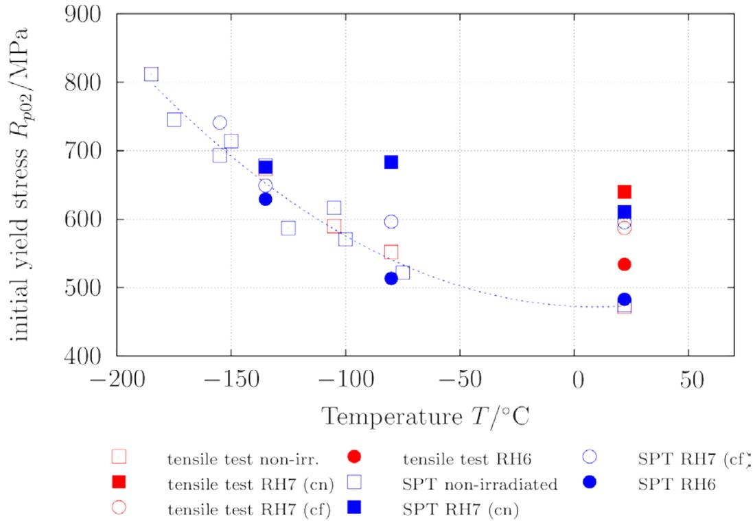
Figure 1: Initial yield stresses identified from the SPT (material JFL; irradiation levels: non-irradiated, RH6, RH7cf/cn)
