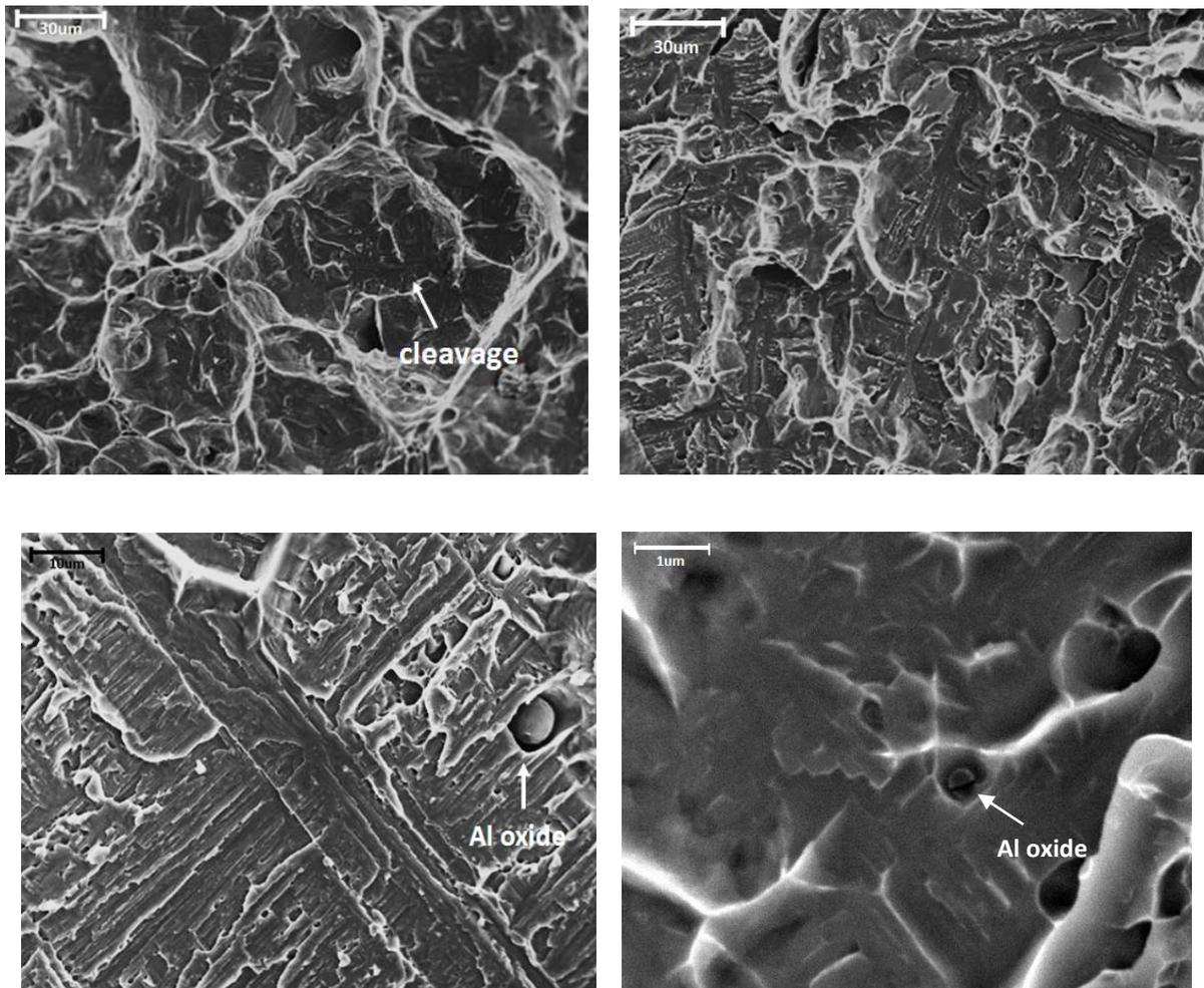
Figure 3 Influence of temperature on fracture in duplex stainless steel, (a). At  $-75^{\circ}\text{C}$ , impact toughness 46J, (a). At  $-130^{\circ}\text{C}$ , impact toughness 14J, (c). Enlarged cleavage fracture at  $-75^{\circ}\text{C}$ , (d). Enlarged cleavage in weld metal at  $-100^{\circ}\text{C}$ , a cracking inclusion is a Griffith crack.
