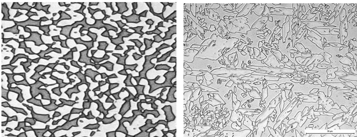
Figure 1 Typical microstructure of SAF 2507; (a). Base material, X200, (b). Weld metal.
