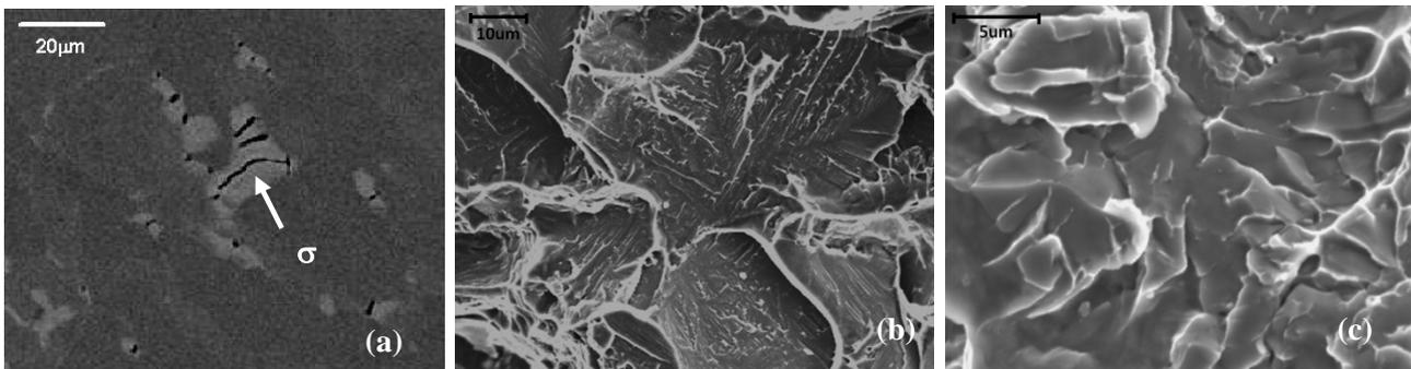
Figure 6 Influence of sigma phase on cleavage in duplex stainless steel at RT. (a). Cracking of sigma phase, (b). Cleavage fracture in the material with about 1% sigma phase, (c). Cleavage fracture in the material with about 10% sigma phase.
