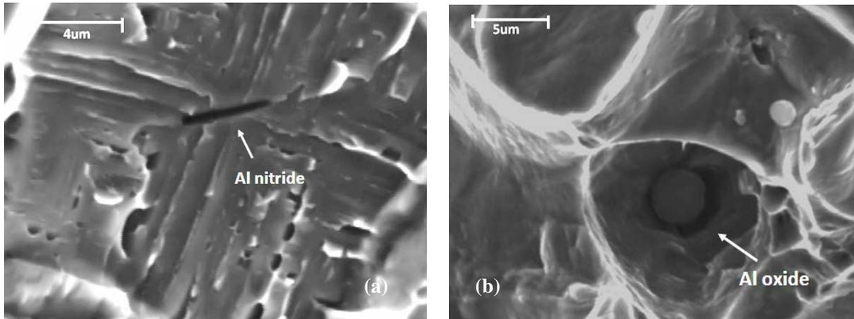
Figure 7 Influence of precipitate and defect on cleavage in duplex stainless steel. (a). Al nitride, (b). Al oxide at  $-130^{\circ}\text{C}$ .
