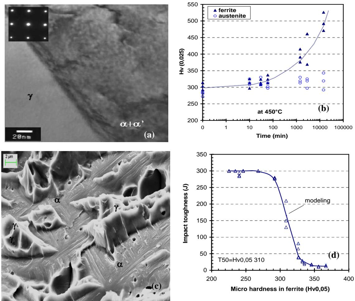
Figure 4 Influence of spinodal decomposition on DBT of DSS, (a). Formation of cluster, (b). Influence of spinodal decomposition on the hardness of individual phases, (c). Fracture, (d). Correlation between hardness and impact toughness;  $\alpha$  is the ferritic phase or Fe rich cluster,  $\gamma$  is the austenitic phase,  $\alpha'$  is the Cr rich cluster or phase.
