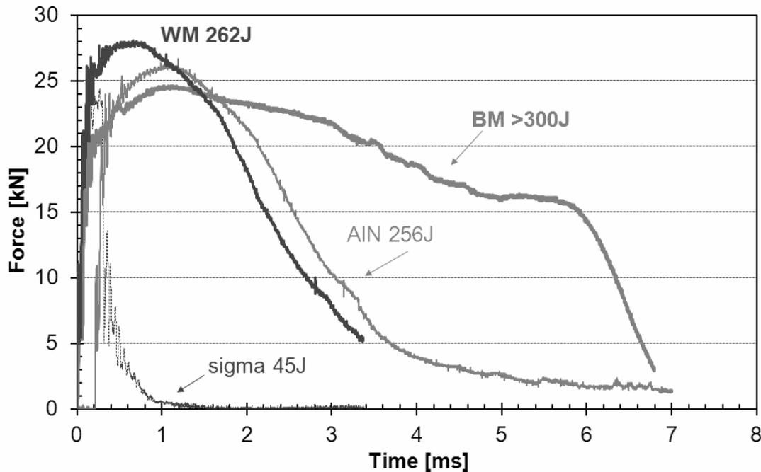
Figure 5 Force versus time curves from the instrumental impact toughness testing for SAF 2507 material with different conditions
