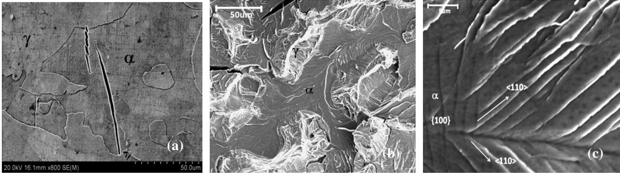
Figure 8 Cleavage initiation and propagation in hydrogen enriched duplex stainless steel,  $\gamma$  –austenite,  $\alpha$ -ferrite.
