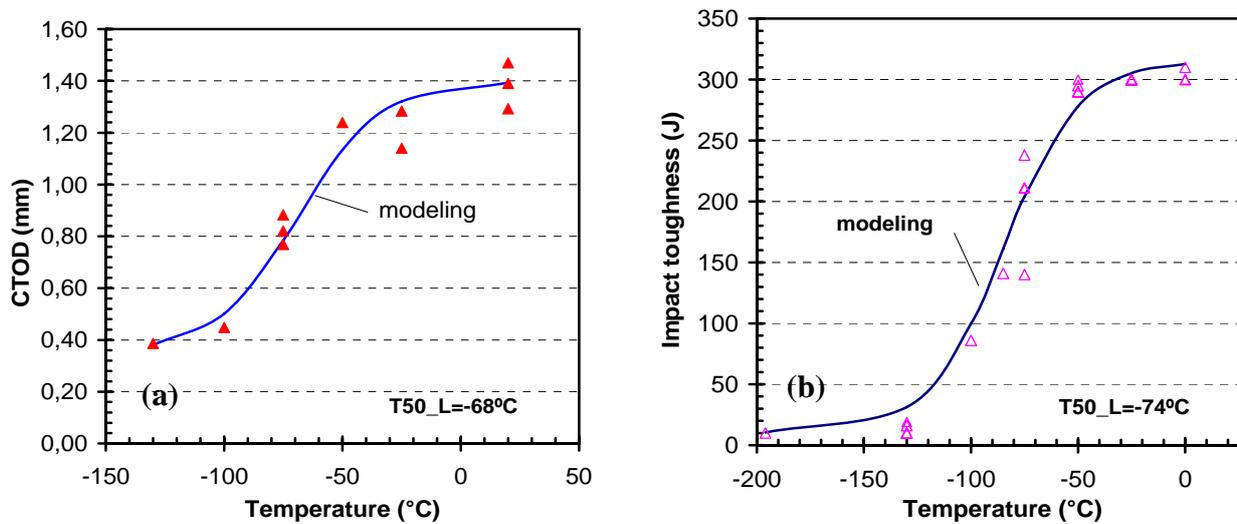
Figure 2 DBT behavior of UNS S32750 SDSS, (a). CTOD (b). Impact toughness.
