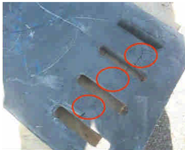
Figure 4. Photo UHPC2.5 specimen cracks after 6-meter high free falling test
