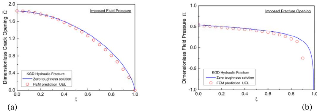
Figure 5. Zero-toughness case: (a) Imposed pressure; and (b) Imposed opening
