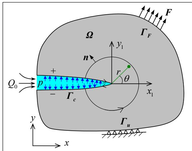
Figure 1. A two-dimensional domain containing a hydraulic fracture
