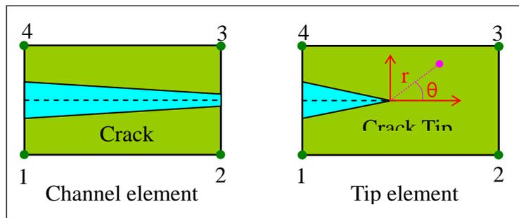
Figure 3. 2-D 4-node plane strain hydraulic fracture elements
