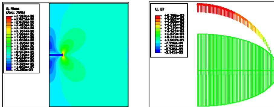
Figure 6. Stress and crack opening profile of a center-cracked tension plate
