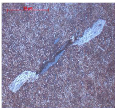
Figure 12 Comparison between wings in rolling contact fatigue and push pull gigacycle fatigue in a bearing steel
