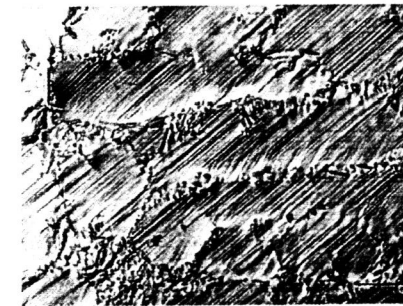
Fig. 7: Nomarski-contrast micrograph showing the interaction between slip bands and Si particles in cell boundaries in a sample with large cell size. DAS: 56 μm. Applied strain: 1.4%.
