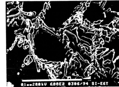
Fig. 5: Deep-etched sample showing the structure of the dendritic cell boundaries in a sample with large cell size. DAS: 40 μm. Unmodified alloy.
