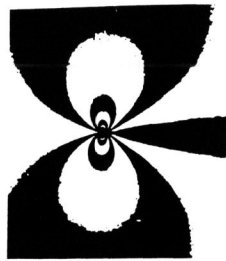
Fig. A-2 Mode I fringe pattern prior to Post and Tardy refinement
