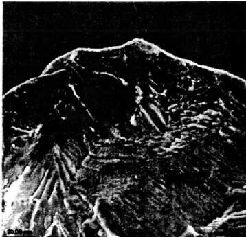
Figure 9: SEM picture of an fatigue initiating defect. Note folds and laps at corner.
