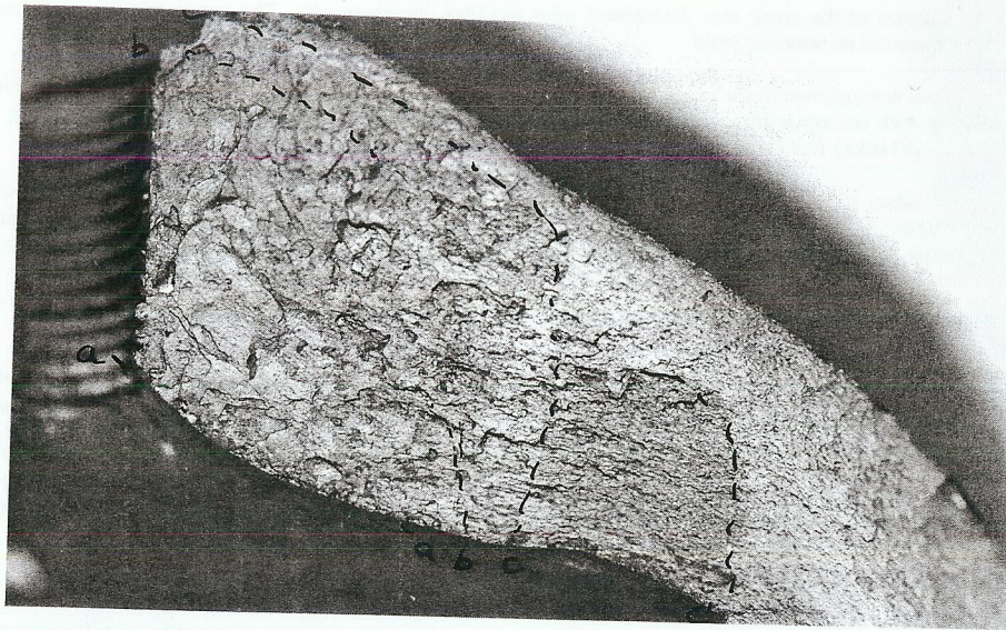
Figure 3 The fracture surface on one of the four fractures on cylinder B. The photograph has been marked to high-light beachmarks caused either by damage during hydro tests of the cylinder or indicating changes to the crack growth mechanism. Some growth stages might leave no clear beach mark.
