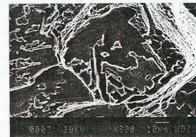
Fig. 10. Beta raft upon underlying alpha plate, exposed via \alpha/\beta interface cracking.
