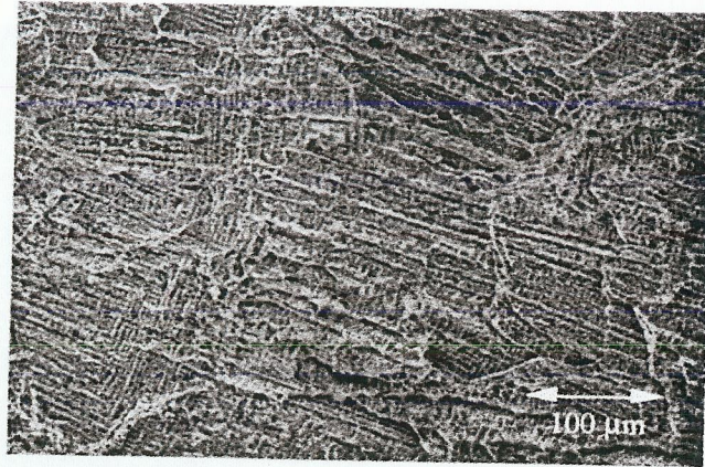
Figure 5 Fracture surface of weld metal in Figure 4. The fracture appearance is low ductility dimples with fracture along cell interfaces.
