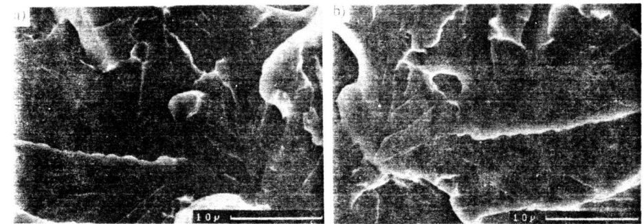
Figure 11. Matching cleavage facets for steel 2 showing a debanded MA particle.
