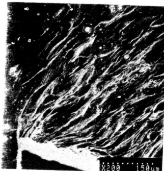
Figure 2. Slip bands over the rake face of cutting tool, when cutting pure iron. (SEM)
