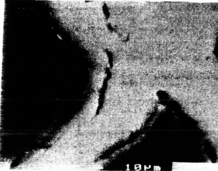
Fig.4 - Voids nucleated near SiC particulates
