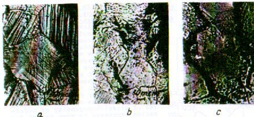
Fig.7. Micropicture of deformation in the zone of destruction of the heat-proof nickeliferous alloy at 750^{\circ}\text{C} , speed of deformation 1 \cdot 10^{-6} \text{ s}^{-1} : a-the 1st, b-the 2nd, c-the 3d regimes of heat treatment, correspondingly.
