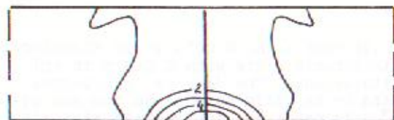
Fig. 2. Distribution of isolines of crack specific volume in ceramic plate after 2 and 4 \mu\text{s} after interaction with velocity of 1000 m/s.
