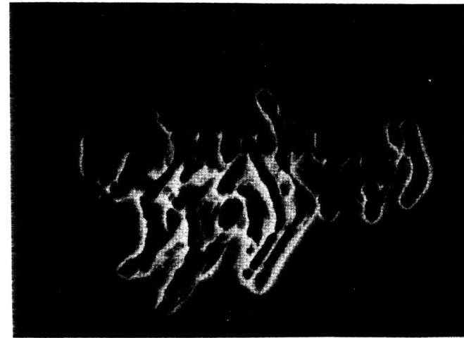
Fig. 6 Micrograph of traces of dislocations during fast fracture at a temperature higher than the BDT temperature.
