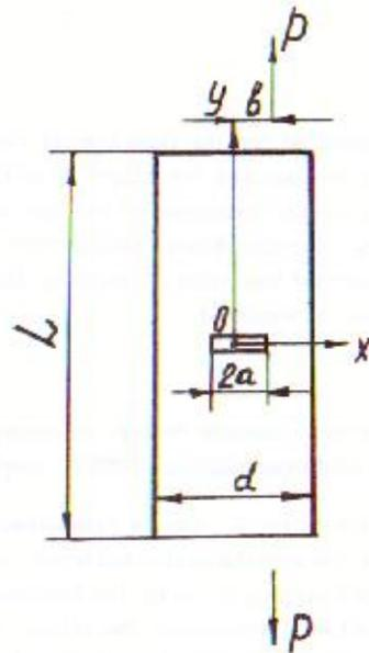
Fig.1. Diagram of the cracked specimen.
