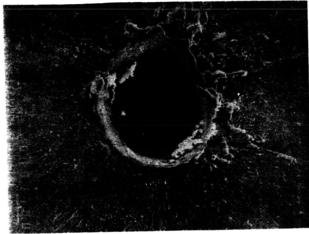
Figure 3.- SEM micrograph - fracture (quenching + artificial aging).
