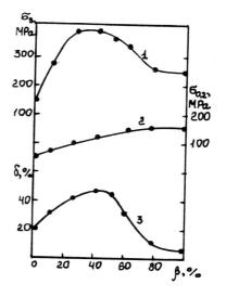
Fig. 1 Mechanical properties of palladium as a function of the completeness of  $\alpha \rightarrow \beta$  transformations: 1-ultimate strength, MPa; 2-yield limit, MPa; 3-relative elongation, %.
