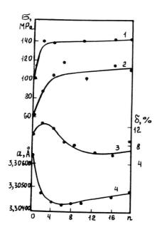
Fig. 2 Influence of the HPN - treatment on the mechanical properties of the NbHo.o3 and the lattice parameter of its matrix ( $\alpha$ -phase): 1- $\sigma_{\rm B}$ : 2- $\sigma_{\rm O}$ : 3- $\delta$ ; 4- $\sigma_{\rm C}$ .
