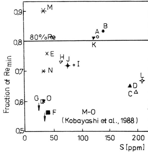
Fig. 2. SSC susceptibility in dependence on the sulphur content
