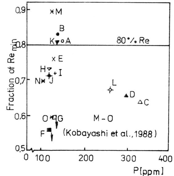
Fig. 3. SSC susceptibility in dependence on the phosphorus content
