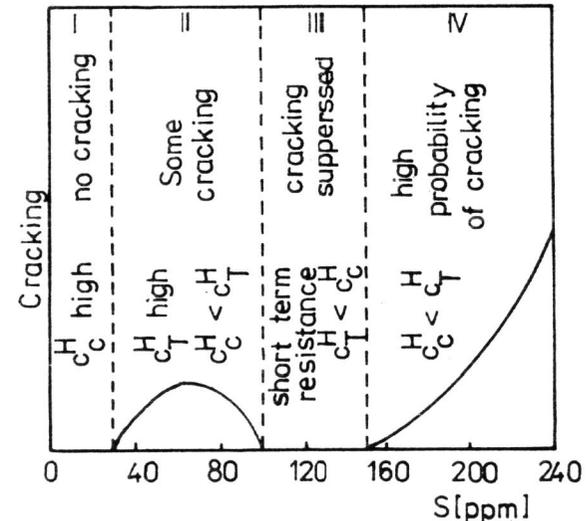
Fig. 4. Frequency of cracking in SSC tests in dependence on the sulphur content
