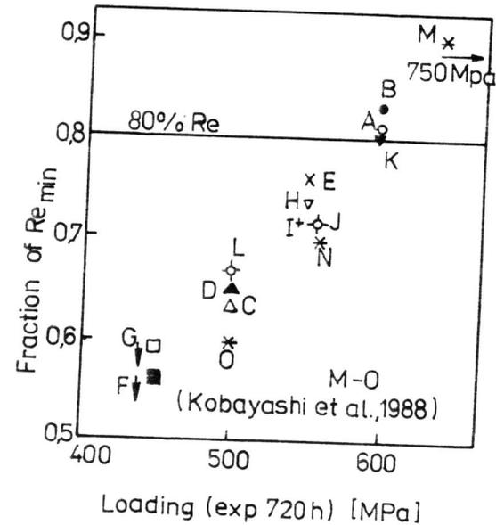
Fig. 1. SSC susceptibility in dependence on exposure of 720 hours
