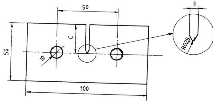
Fig.1. Shape and dimensions of specimens
