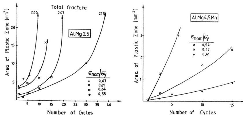
Figs.3 and 4. The area of plastic zones as a function of the number of load cycles.
