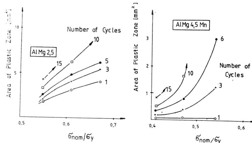
Figs.5. and 6. Plastic zone sizes as a function of the load levels.
