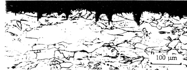
Fig.4.- Optical micrograph showing lateral secondary cracks starting in the hydride layer in Ti Gr-2 tested at 2.4 \times 10^{-7} \text{ s}^{-1} strain rate with -1500 mV (SCE) cathodic polarization.
