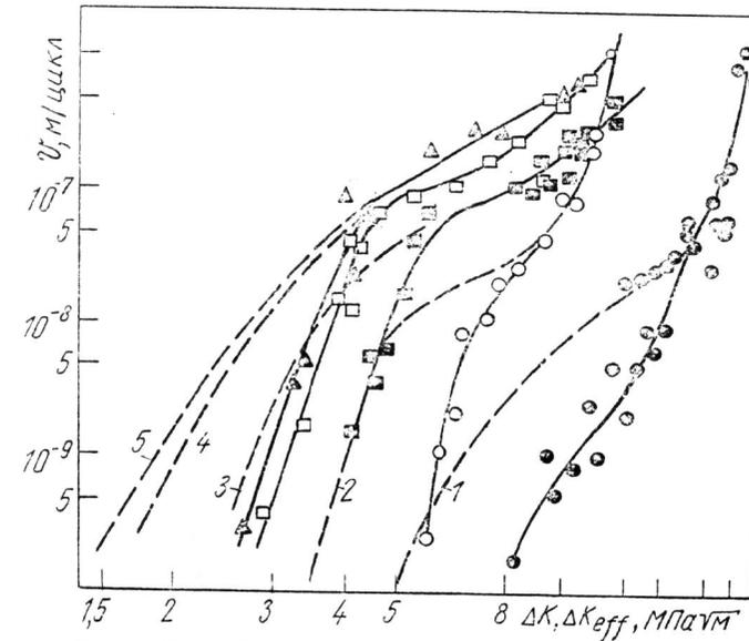
Fig. 2.  $v - \Delta K$  (symbols) and  $v - \Delta K_{eff}$  (lines) dependences for HK-40 steel in hydrogen at different temperatures: 20°C (●,1); 200°C (○,2); 400°C (■,3); 600°C (□,4); 800°C (▲,5).
