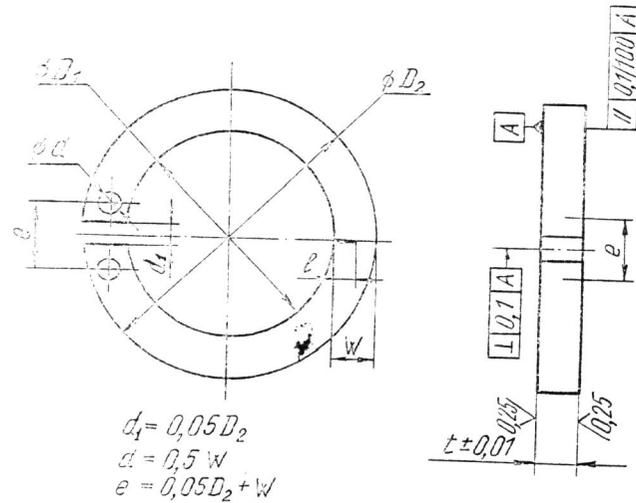
Fig. 1. A sketch of ring-type specimen for the crack resistance testings at high temperature.
