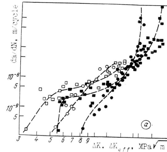
Fig. 3. Fatigue fracture kinetic diagrams of HK-40 steel in the air (■,□) vacuum (▲,Δ) and hydrogen (●,○) at temperatures: a - 20°C; b - 200°; c - 400°; d - 600°; e - 800°C. Dark dots correspond to nominal SIF values, light - to effective.
