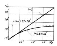
Current loading effect on fatigue of copper specimens. (The point indicated the average value and 95% confidential interval of smooth specimen lives).
