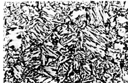
Fig.3 A typical optical micrograph of a dual phase steel
