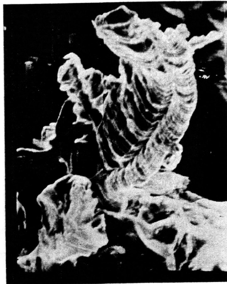
Fig.3 A shy shylock in the metallic society- an unusual art of hydrogen embrittlement attack in the form of a botanical leaf. X 400
