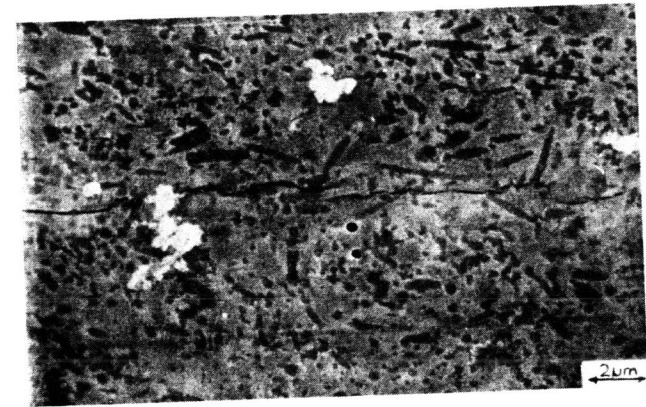
Fig. 6 : SEM photograph (2000x) showing both deflection and bridging
