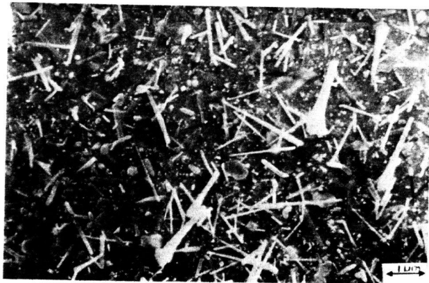
Fig. 5 : Scanning Electron Micrograph (1000x) of polished and etched surface showing uniform distribution of SiC whiskers throughout the alumina matrix
